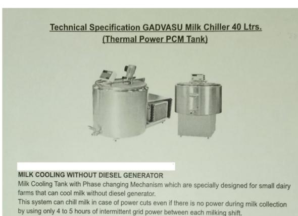
By eliminating diesel, Thermal Power Tanks provide the most cost effective way of collection centers where grid power is erratic.
